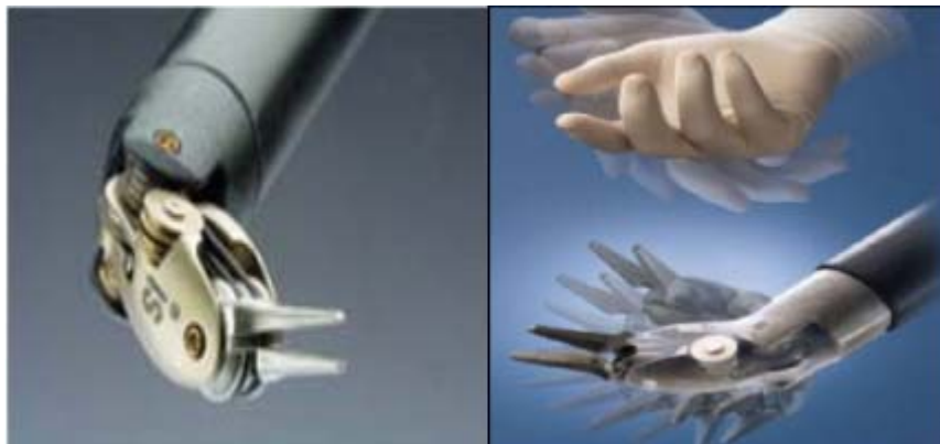
Fig. 2: Endowrist-instrument specific daVinci™ cu 7 grade de libertate
