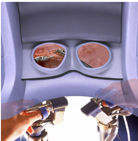
Fig. 3 Hands position corresponds to instrument tip orientation
