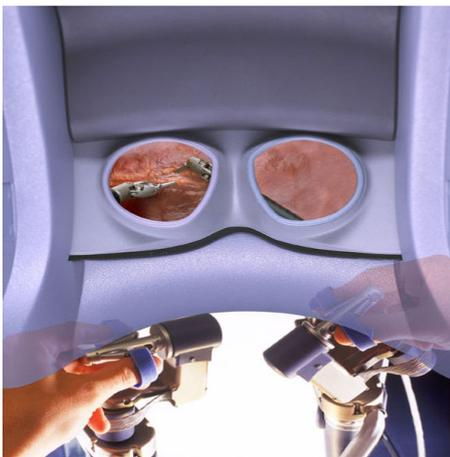
**Fig. 3 Hands position corresponds to instrument tip orientation**
